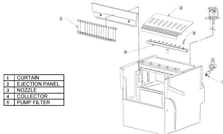
**CAUTION:** IT IS VERY IMPORTANT WHEN REPLACING THE CONTAINER THAT THE NOZZLES ARE PERPENDICULAR, AS IF TWISTED, THE EXTERNAL CUBES COULD RUN OUT OF WATER.
