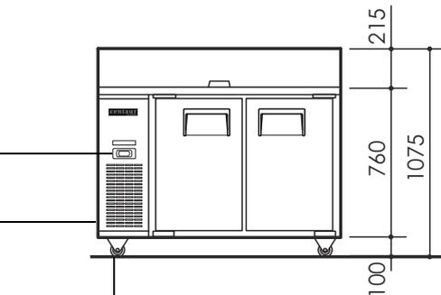
Swivel castors (front locking) or four adjustable legs (100-160mm)
