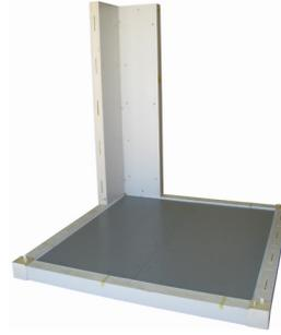
4. Continue fitting back and side wall panels, working from the back towards the front of the room. Use fast-fit inserts to align wall panels correctly and lock in place with cam locks.
