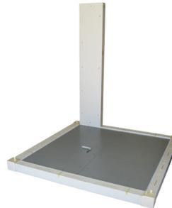
2. Fit a wall panel edge piece. Use fast-fit inserts to align and lock in place with wall panel cam locks. Ensure the top edge of the edge piece is level with the top of the wall panel.
