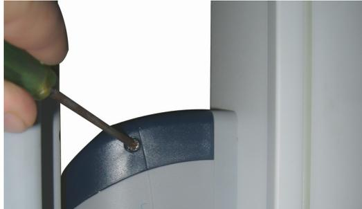
2. Close the door and loosen the two adjustment screws.
