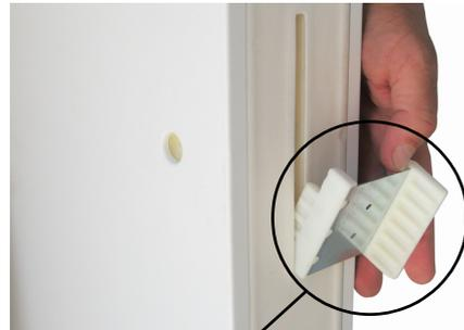
7. Lift the ceiling panel/s onto the room walls, hang using the ceiling supports and lock into place. If fitting multiple ceiling panels, fit the rear panel first and work forward.
