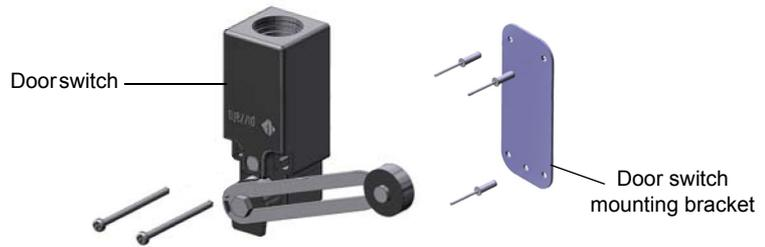
**To install the sliding door switch and activator bracket**
