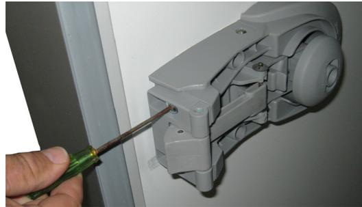
3. Move the lock section of the handle in or out as necessary to align correctly.
