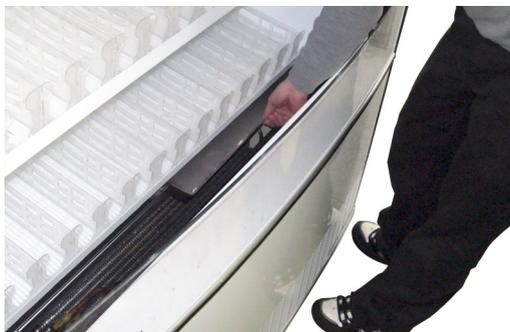
3. When refitting, ensure the return air grille and both spill trays are in place and fitted correctly. See page 9 for correct configuration.
