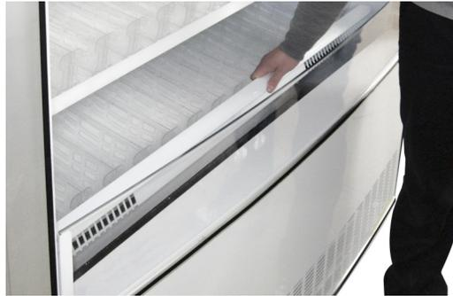
2. Remove the front panel by locating and unclipping the two bottom brackets (can be felt at the bottom of the front panel), and lift the front panel up and off the cabinet.
