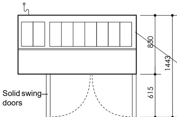
7 x 1/3 150mm deep pans (refrigerated) & 2 x 1/3 65mm deep pans (ambient) with 3 pan lids. Pan lids must be in place when pans not in use.
