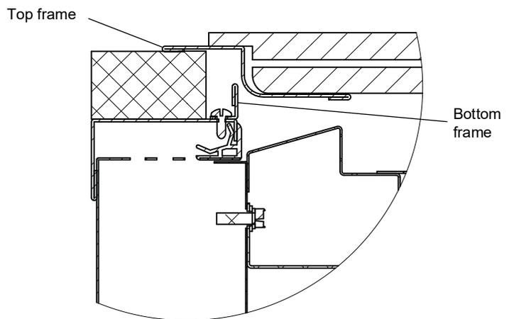
5. Rotate the top frame into position on the customer's benchtop, taking care not to damage the heat element wires. The top frame will nest within the bottom frame.
