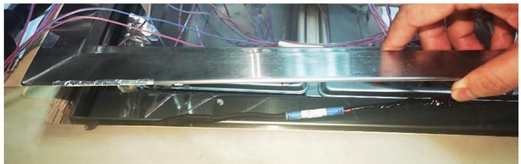
6. Apply glue or sealant around the edge of the drop-in collar to stop food getting trapped after the collar has been installed.
