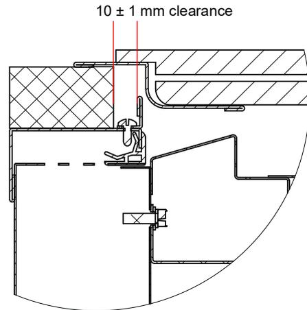
3. If you removed the collar's bottom frame, refit this to the cabinet top by mounting it in its original position and securing with the self-tapping screws.
