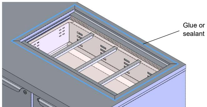
7. Use weights to hold the top frame in position while the glue or sealant cures.
