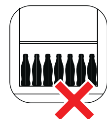
Cabinet Floor Do not load product on the cabinet floor. Use the shelves.
