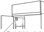
The rating label is located inside the cabinet at the top front of the left or right side wall.
