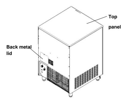
C) Remove the back metal lid and the top panel (if it need be to make easier the cleaning OPErations).
