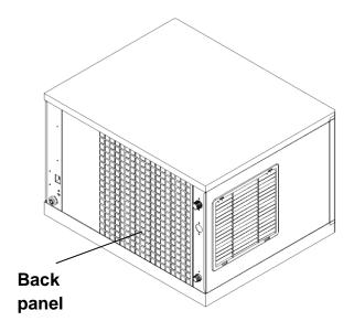
3) Clean condenser using a vacuum cleaner, soft brush or low pressure air. Clean from top to bottom, not side to side. Be careful not to bend the condenser fins.
